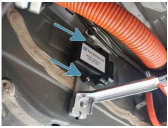
4. Fit the supplied wiring harness making sure no cable strain exists and all connectors are clipped firmly in place. Fix wiring harness in place to the top of the HV Cable using the supplied wiring support and 2 x cable ties as per below images, trim off cable tie excess using side cutters taking care not the damage any wiring.
