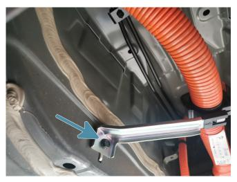
2b. Align the mounting bracket and fix in place using a thread locking compound with the supplied M6 button head screw and washer at the bottom and retaining clip up top.
