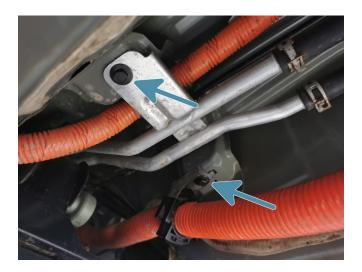
3b. Align the mounting bracket and fix in place using the 2x supplied M6 button head screws and washers on either side as shown below
