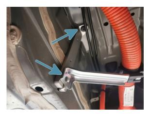
2. Mount Charge Controller to the bracket using a thread locking compound with the 2 x supplied M5x16mm screws ensuring the translator connector is facing the rear of the vehicle.
