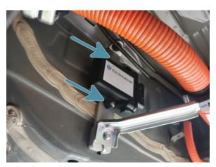
3. Fit the supplied wiring harness making sure no cable strain exists and all connectors are clipped firmly in place. Fix wiring harness in place to the top of the HV Cable using the supplied wiring support and 2 x cable ties as per below images, trim off cable tie excess using side cutters taking care not the damage any wiring.
