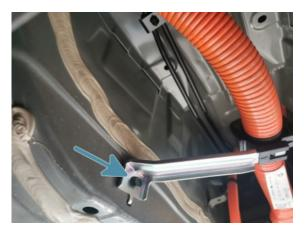
1b. Align the mounting bracket and fix in place using the supplied M6 button head screw and washer with thread locking compound at the bottom then insert the retaining clip up top.
