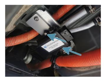
5. Fit the supplied wiring harness making sure no cable strain exists and all connectors are clipped firmly in place. Fix wiring harness in place to the top of the HV Cable using the supplied wiring support and 2 x cable ties as per below images, trim off cable tie excess using side cutters taking care not the damage any wiring.
