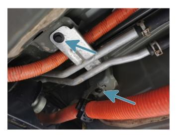
3b. Align the mounting bracket and fix in place using the 2x supplied M6 button head screws and washers on either side as shown below
