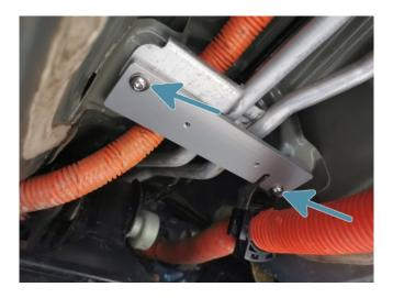
4. Mount Battery Translator to the bracket using the 2 x supplied M5 button head screws ensuring the translator connector is facing the rear of the vehicle.
